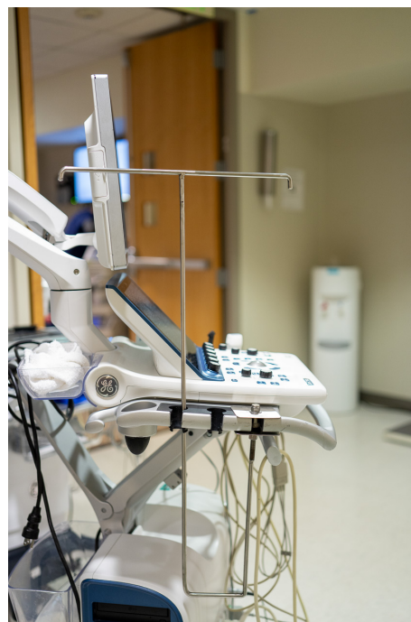
Figure 2. Echo shield component parts (left panel) and installed on echo machine (right panel). The right panel shows the echo shield stowed in transport position (tall support rod stowed in neighboring probe-holder hole).
