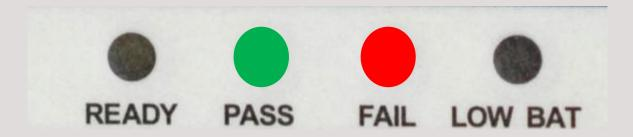
If Leakage Test fails, take out of circulation and call service representative
