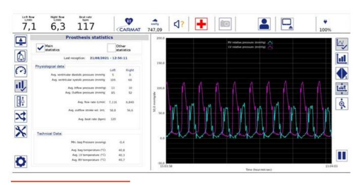
FIGURE 6: CARMAT CONSOLE DISPLAY WITH AVERAGES OF FLOW AND PRESSURE (LEFT PANEL) AND REAL-TIME LEFT VENTRICULAR (PURPLE) AND RIGHT VENTRICULAR (TURQUOISE) PRESSURE CURVES (RIGHT PANEL)
