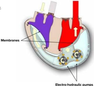
FIGURE 2: SCHEMATIC OF THE INSIDE OF THE CARMAT TOTAL ARTIFICIAL HEART. BOVINE PERICARDIAL MEMBRANES SEPARATE EACH VENTRICLE INTO A BLOOD COMPARTMENT AND SILICON OIL COMPARTMENT, AND THE ENTIRE SYSTEM IS ENCASED IN A POLYURETHANE SAC WITH SILICON OIL. TWO ELECTRO-HYDRAULIC PUMPS MOVE THE BOVINE PERICARDIAL VENTRICULAR MEMBRANES WITHIN THE SILICON OIL TO SIMULATE DIASTOLE AND SYSTOLE.
